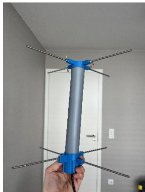
Figure 5: Our home-made turnstile antenna
